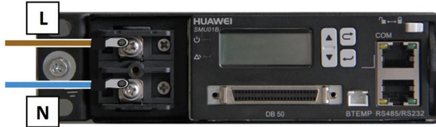
Figure 4-11 Connecting the single-phase AC input power cable
