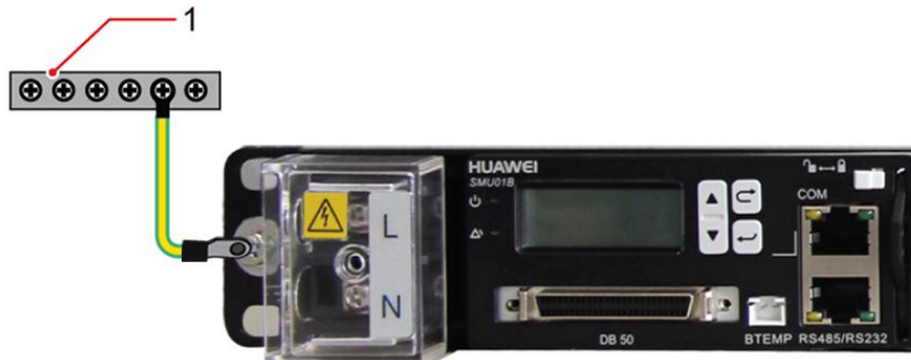
Figure 4-5 Connecting the ground cable
